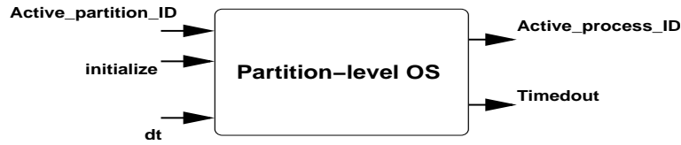
Fig. 11. Interface of the partition level OS model.
