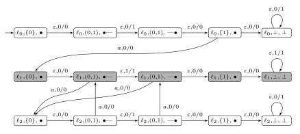
**Fig. 3.** The corner-point abstraction  $\mathcal{A}_{cp}^F$  of  $\mathcal{A}$  represented Fig. 1
