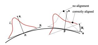
Fig. 6. Rotation  $\mathbf{R}_i$  aligns the coordinate frame at  $\mathbf{p}_i$  with that at  $\mathbf{p}$  to make interpolation possible.
