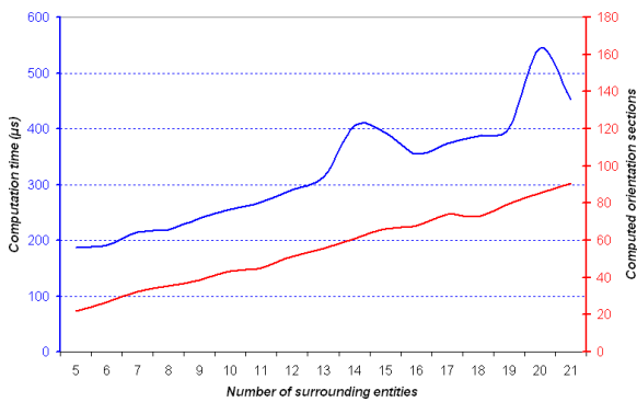
Figure 11: Solution Performance. The blue curve plots the computation time required for solving one interaction according to the number of neighbor entities taken into account. The red curve plots the number of orientation sections created in order to compute the solution. From these plots, it is possible to compute global performances with respect to the density of people.
