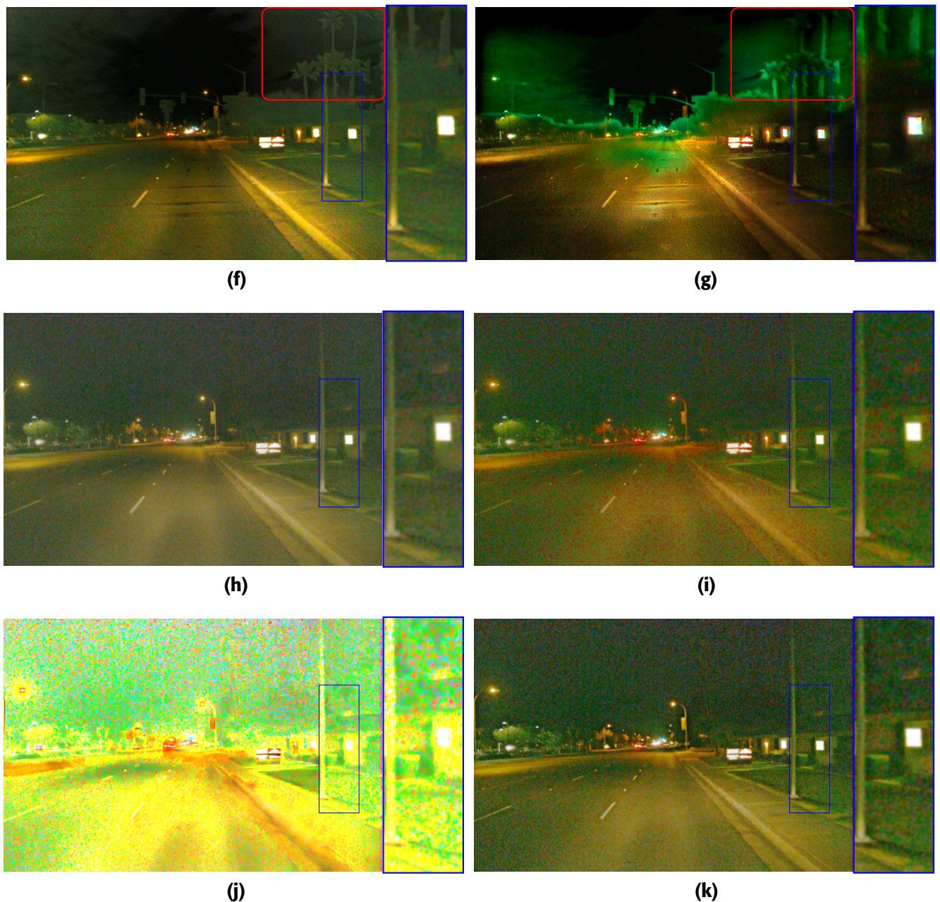
FIGURE 9. Second part of the qualitative comparison between the restoration methods applied to the input image Fig. 9a and the state-of-the-art approaches. Fig. 9f EnlightenGAN [25] and Fig. 9g EnlightenGAN fine-tuned on the Waymo dataset [25] hallucinates trees at the top of the image as shown in the red squares. Applying gamma corrections in the RGB and HSV spaces leads to the outputs illustrated in Figs. 9h and 9i with an undesirable "fog" effect whitening the image. Fig. 9j LIME [13] and Fig. 9k Zero-DCE [31] amplify the noise in the darkest parts of the image.
