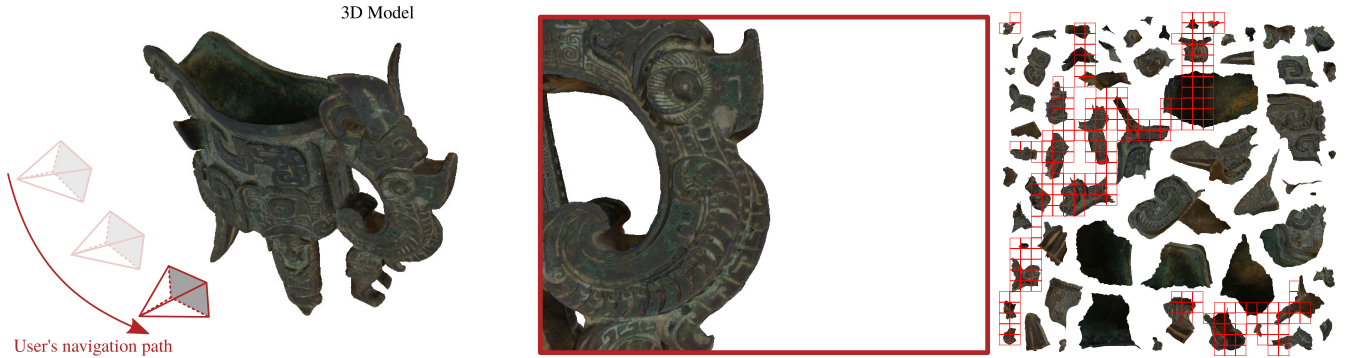
Fig. 2. Example of user's navigation around the 3D model (left), what he observes at a given instant (center), and the corresponding visible blocks \mathcal{V} (in red) in the atlas (right). For better visibility of the blocks, the black background area is turned into white in the atlas.
