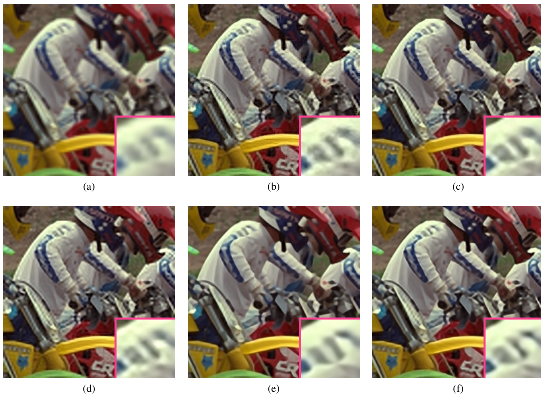
Fig. 9. Comparative results with zoomed-in areas for Bike magnified by a factor of 3. The methods considered are: (a) Bicubic interpolation, (b) LLE-based NE, (c) NN NE, (d) Sparse SR, (e) Pyramid, (f) Proposed.
