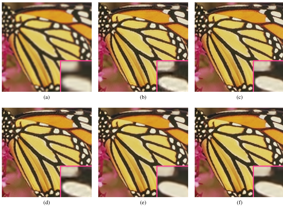
Fig. 8. Comparative results with zoomed-in areas for Butterfly magnified by a factor of 3. The methods considered are: (a) Bicubic interpolation, (b) LLE-based NE, (c) NN NE, (d) Sparse SR, (e) Pyramid, (f) Proposed.
