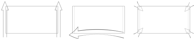
Figure 7: Our storyboard interface rely on a set conventions to describe different types of camera motions. Examples are given for (Left) a dolly up, (Center) a Pan to the left and (Right) a dolly in.
