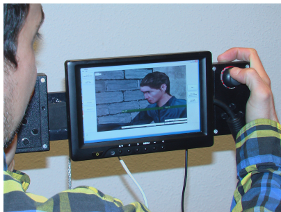
Figure 1: Our custom-built hand-held virtual camera device with dual handgrip thumbsticks, buttons, and 7-inch LCD touch-screen.
