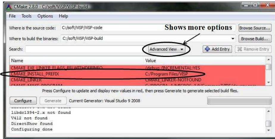
Figure 2: This CMake snapshot shows where to set the CMAKE_INSTALL_PREFIX variable specifying the directory where ViSP will be installed after the build. By default, this variable is set to C:/Program Files/VISP . As shown Fig. 10, this snapshot shows also the location of the menu that allows to print more advanced options like the location of third party headers and libraries.
