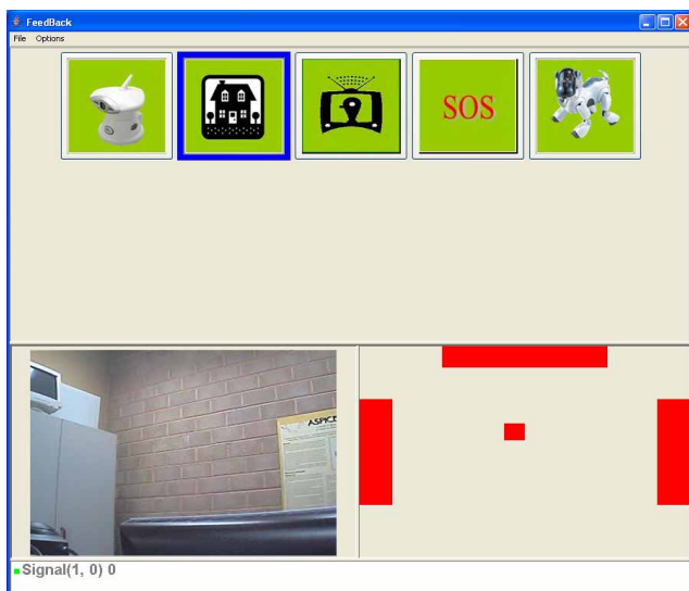
Fig. 2 Appearance of the feedback screen. The Feedback application has been instructed to divide the window into three panels. In the top panel, the available selections (commands) appear as icons. In the bottom right panel, a feedback stimulus by the BCI (matching the one the subject has been training with) is provided; the user uses his learnt modulation of brain activity to move the cursor at the center to hit either the left or the right bars – in order to focus the previous or following icon in the top panel – or to hit the top bar – to select the current icon. In the bottom left panel, the Feedback module displays the video stream from the video camera that was chosen beforehand in the operation.
