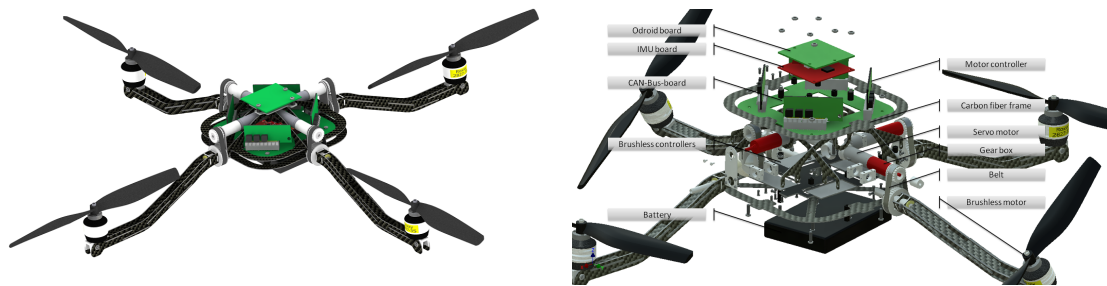
FIGURE VII.7: CAD image of the second-generation prototype with improved mechanics, actuation system, electronics and an overall reduced mass and inertia
