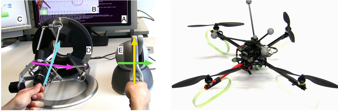
FIGURE V.14: Experimental setup. a) Software components of the framework and input devices: A) TeleKyb; B) SwarmSimX; C) Matlab; D) Omega.6, used to command changes of scale (magenta) and rotations (cyan); E) Phantom Omni, used to command translations along \bar{X}_{\mathcal{W}} (yellow) and along \bar{Y}_{\mathcal{W}} (green). b) The quadrotor used for the experiments.
