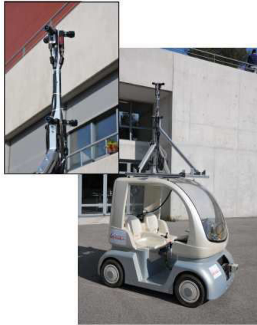
Figure 3.12: Spherical RGBD outdoor acquisition system
