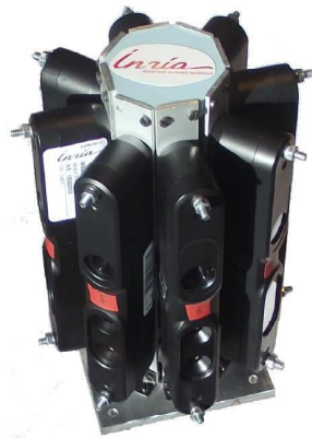
Figure 3.15: Multi RGBD indoor acquisition system comprising of 8 Asus Xtion Pro live sensors
