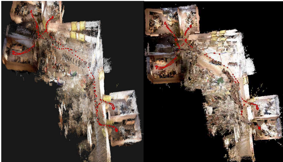
Figure 5.5: Reconstruction comparison with Inria Kahn dataset. Left: No fusion ,Right: fusion with algorithm 2
