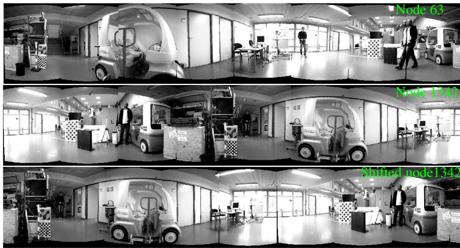
Figure 4.20: Top and centre: Illustration of loop closure between nodes 63 and 1342. Bottom: recovered rotation using outlined SSD technique.
