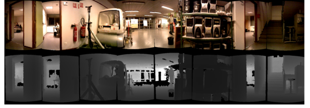
Fig. 6. Omnidirectional RGB and depth images acquired by our RGB-D camera rig.
