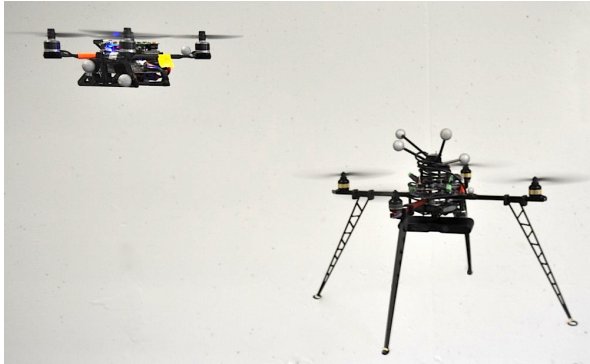
Fig. 3: The quadrotors used for the evaluation: Nano+ from kmel (left) and a MK-Quadro from MikroKopter (right).
