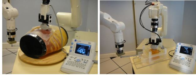
Fig. 3. Experimental setup with the abdominal (left) and gelatin-made (right) phantoms.
