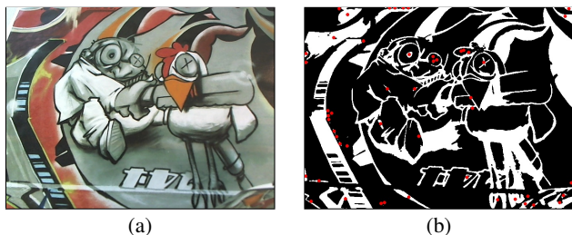
Figure 3: Applying word region detector [21] to Figure 1(a). Binarization by adaptive thresholding was applied to (a) an input image. (b) Few keypoints were extracted from segmented regions because most of the extracted regions were connected.
