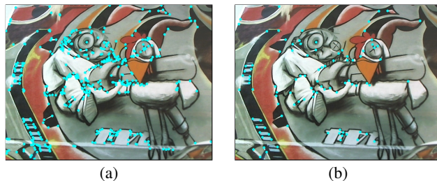
Figure 4: Keypoint selection. FAST was applied to Figure 3(a). (a) 427 keypoints were extracted in total. (b) 100 keypoints were extracted by setting the minimum distance as 10 pixels and the maximum number of keypoints as 100.
