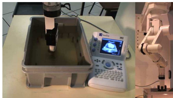
Fig. 8. Experimental setup consisting of a 6-DOF medical robot arm (right), a 2-D US probe transducer, and a water-filled tank.
