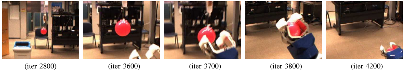
Fig. 7. Experiment B: Key images of the grasping sequence, taken from the embedded (left) camera, and are used during the servo to track the object.
