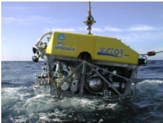
Fig. 1. The Ifremer Victor 6000 underwater ROV (© Ifremer)
