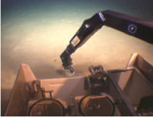
Figure 2: The Victor 6000 six dof manipulator Maestro (© Ifremer)
