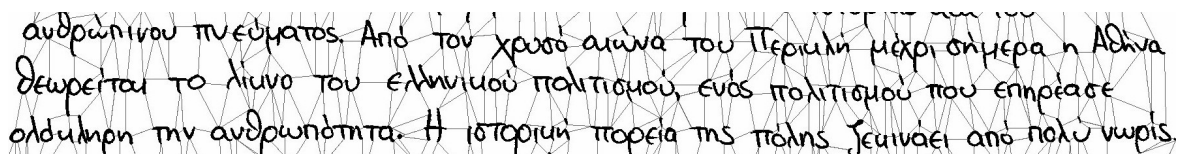
Figure 4. Delaunay graph for distance computation: the vertexes give the distance between pixels of the neighbor connected components
