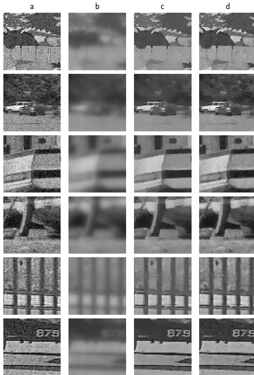
Figure 2: Sample of the results obtained for the 40 images benchmark. (a) Noisy images, (b) restored images with the quadratic model, (c) restored images with the robust model (the IRLS method and the Cauchy estimator), (d) restored images with the robust model (the FAJM method and the Cauchy estimator).
