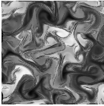
Fig. 4. Velocity constraints and fluid imagery for a two-dimensional flow. Velocity vectors provided by the DNS which have been selected as constraints are superimposed on the image.
