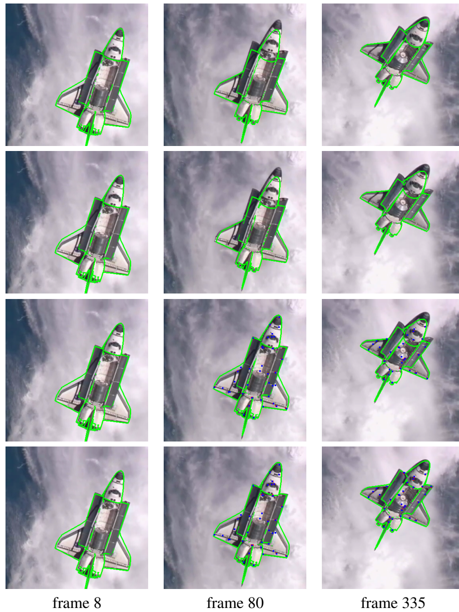
Figure 4.27 – Tracking for the Atlantis sequence with, from top to bottom, [C_0, C_1] , [C_0, C_1, C_3, C_4] , [C_0, C_1, C_3, C_4, C_5] and [C_0, C_1, C_3, C_4, C_5, C_6] , frames 8-335
