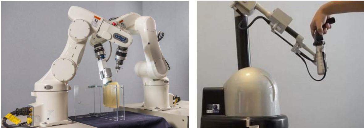
Robotic platform for needle steering: 6-dof robot holding an 3D ultrasound probe, 6-dof robot actuating a flexible needle, Haption Virtuose 6D haptic device.
