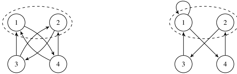
Fig. 1.2 On the left graph P is periodic and G' is aperiodic. On the right graph P aperiodic and G' is periodic.
