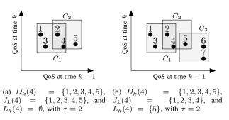
Fig. 4. Splitting the neighborhood of device 4 into  $J_k(4)$  and  $L_k(4)$ .
