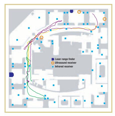
Figure 6. Tracking with anonymous and ID sensors. The blue-shaded circles indicate areas covered by ID sensors such as infrared receivers. Because these sensors provide no information about the person's location in the area, two people in the same area can't be distinguished. Not shown is an additional anonymous sensor, such as a laser range finder, providing accurate location information at a high rate but no information about the persons' IDs.
