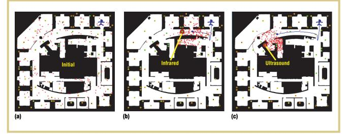
Figure 4. A particle filter for location estimation using infrared and ultrasound sensors: (a) A person wearing an infrared badge and ultrasound tags starts in the upper right corner. (b) After the person moves out of the cubicles, the samples are spread over different locations. (c) An ultrasound sensor detects the person.
