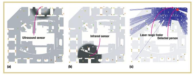
Figure 3. Probabilistic models for (a) ultrasound tags, (b) infrared badges, and (c) laser range finders. The environment is 30 m  $\times$  30 m. In (a) and (b), darker areas indicate higher likelihoods of observing the corresponding measurement. Walls and other obstacles are white because they have zero likelihood. In (c), laser-scan beams, along with a detected person, are blue. The person obstructs the laser beams, thereby causing a "shadow" in the scan.
